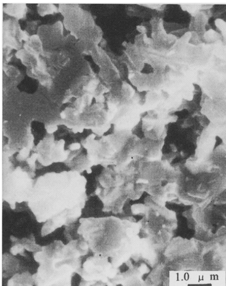
Fig. 7. SEM micrograph of fracture surfaces of sample 2 treated at 1200°C and sintered at 1580°C for 4 h.
