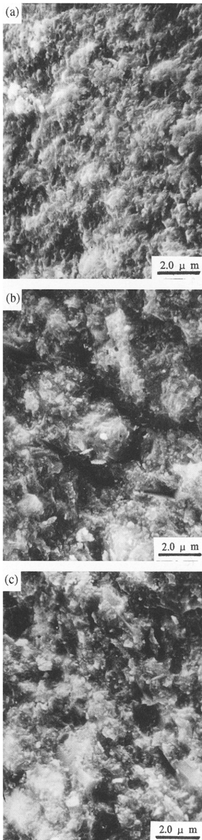
Fig. 11. SEM micrographs of fracture surfaces of samples: (a) sample 3, 1550°C; (b) and (c) sample 1, 1550°C.
